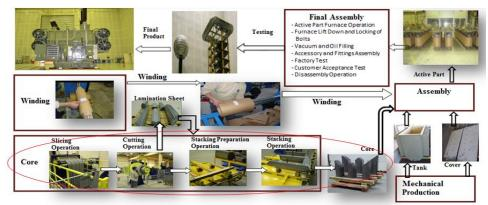
Fig. 5: Summarized production flow chart for magnetic core production.
