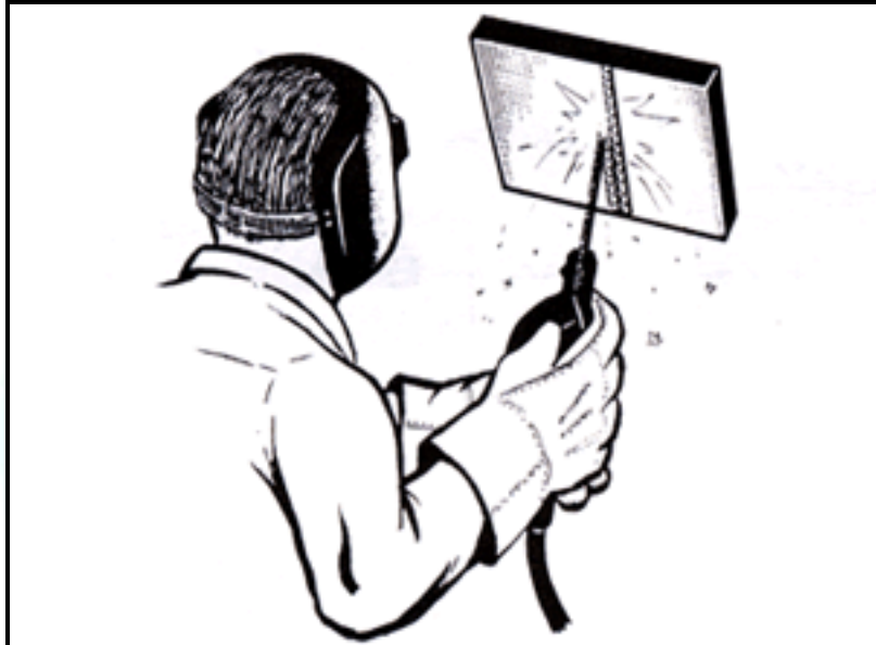
Fig 23. Position yourself for visibility and comfortable electrode manipulation.
