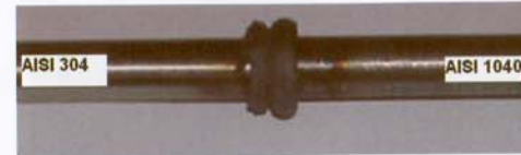
Fig. 2: Photo of welded specimens
